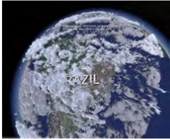
Figure 6: MeteoVis renders volumetric clouds from the GOES Cloud Top Height Data. We shade the clouds based on the relative heights: lower clouds are shaded in a darker color.
