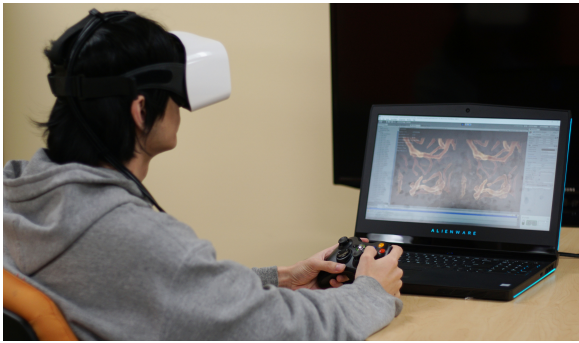
Fig. 4. Our user study set up with gaze-tracker integrated into the FOVE head-mounted display.
