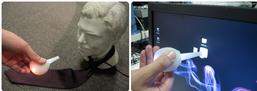
(a) Slurp extracting a digital object from a sculpture (b) Slurp injecting a digital object onto a screen
