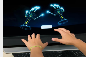
Leap motion (Stereo Infrared camera and IR LEDs for hand tracking)
