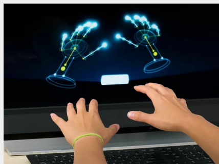
Leap motion (Stereo Infrared camera and IR LEDs for hand tracking)
