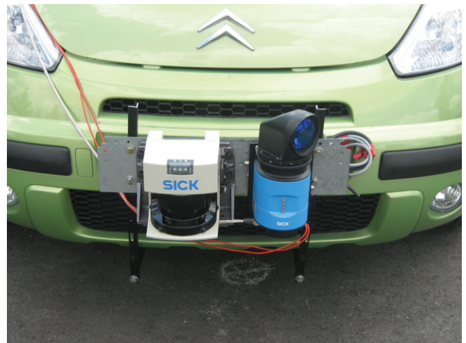
Fig. 2. (Colour online) LMS-291 (left) and LRS 1000 Laser Radar (right).
