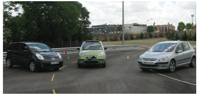
Fig. 1. (Colour online) Test vehicle with radars mounted on the bumper (center), black colored car (left) and gray (silver) colored car (right).
