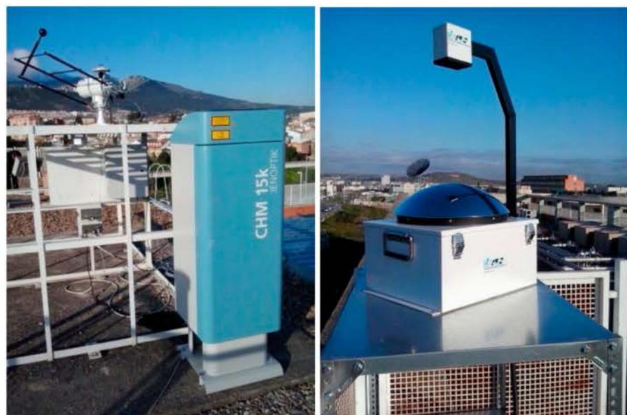
Figure 2. Meteorological station of the University of Jaen. (left) Ceilometer and Sun tracker in the background. (right) The TSI-880 sky camera.
