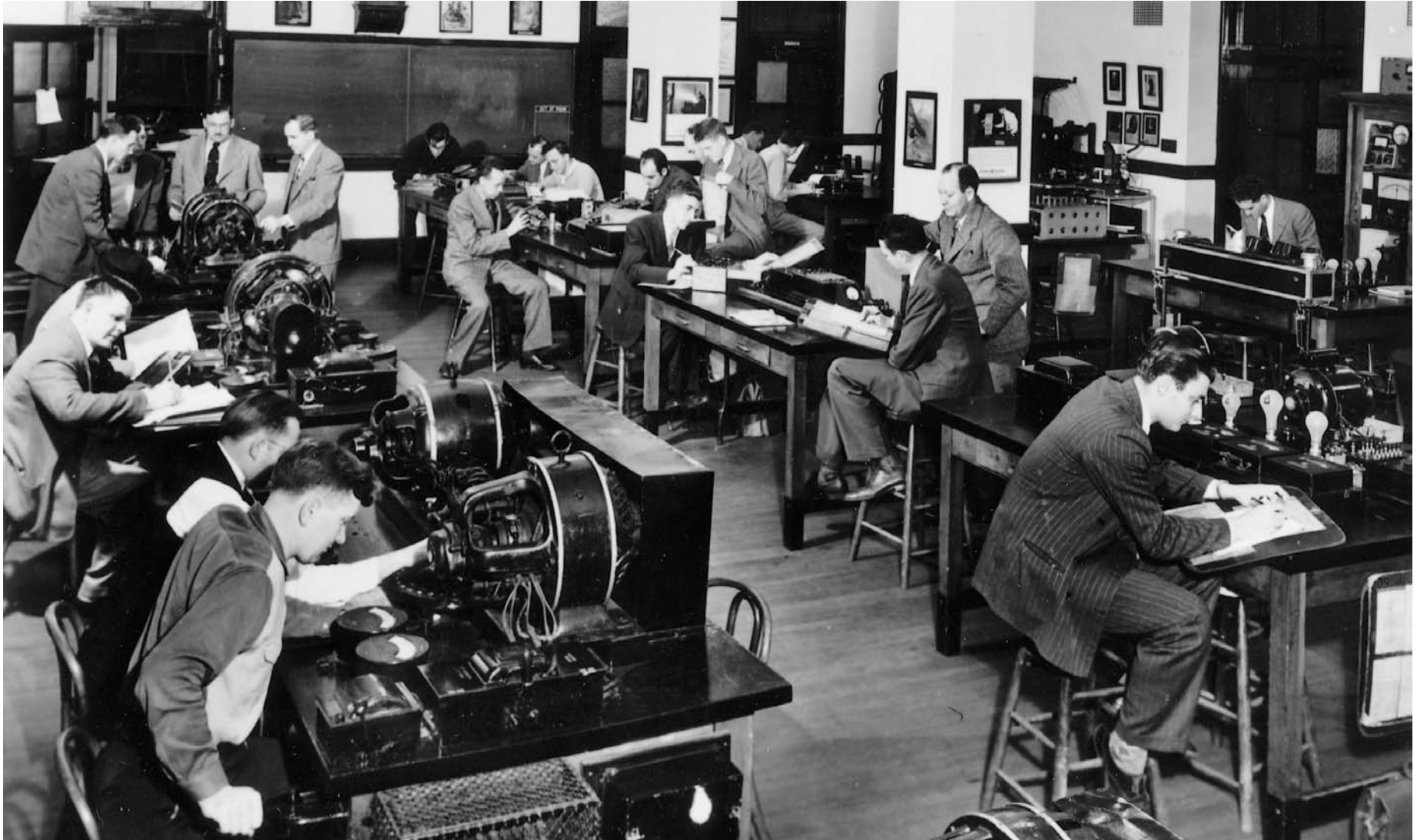
Electrical engineering lab testing motors for voltage and amp meters in the early 1950s, courtesy University Archives.
