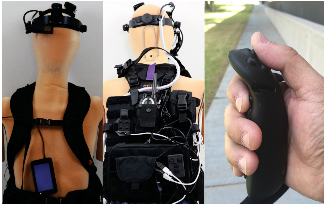
Figure 3. Front (left) and back (middle) views of the wearable computer. The wearable consists of: front: a monocular, see-through HMD with compass and GPS attached and a tethered handheld display; back: interconnects and a notebook computer. View of the chording keyboard, Twiddler (right): players used the thumb to record familiarity and the forefinger to bring up the interface.
