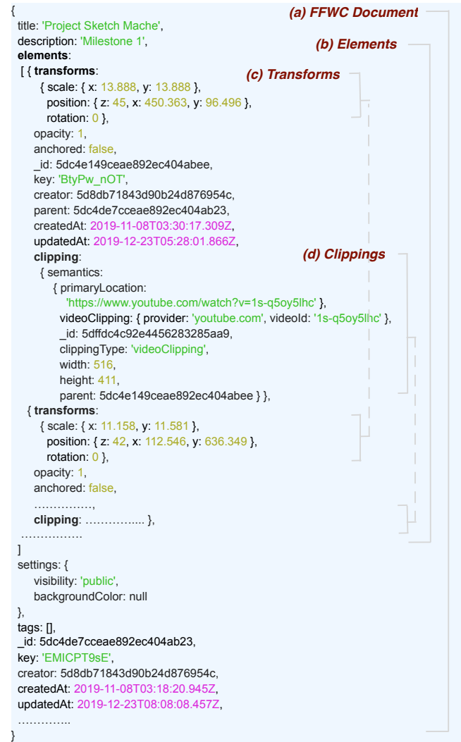
Figure 2: An FFWC document is comprised of properties such as title , description , creator , and a collection of elements . Each element includes a transforms property—with sub-properties position , scale , and rotation —which allows determining the element’s spatial location with respect to the origin. Each element also stores a clipping property, which in turn stores semantics extracted at the time of collecting the element.
