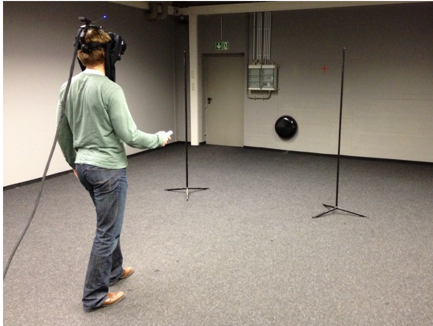
Figure 5.5: Experiment setup: participant walking in the direction of a target displayed at eye height for a distance indicated by the center of two vertical poles.
