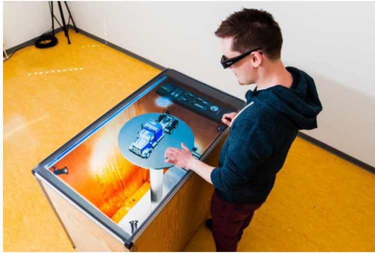
Figure 1.7: User interacting with a virtual scene in a stereoscopic multi-touch tabletop setup using touch-enabled 3D widgets. The widgets in the graphical user interface were rendered with negative parallax of up to 10cm height.
