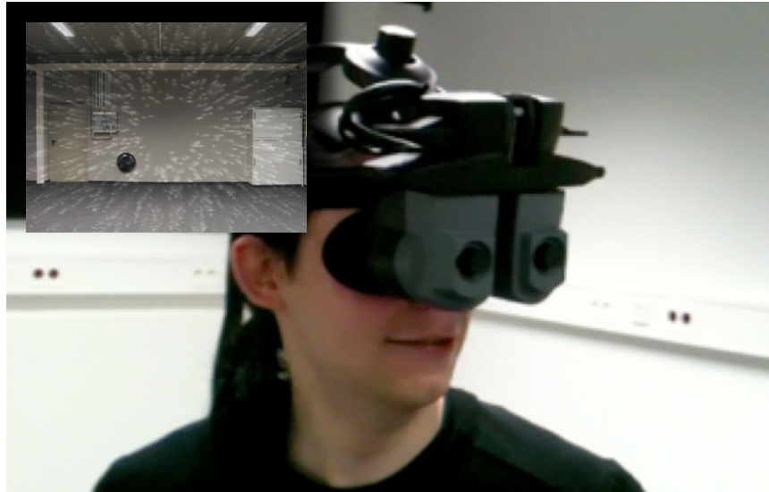
Figure 5.1: Photo of a user wearing a tracked NVIS nVisor MH-60V video see-through HMD. The inset shows an illustration of the resulting expansional optic flow field during forward movements.
