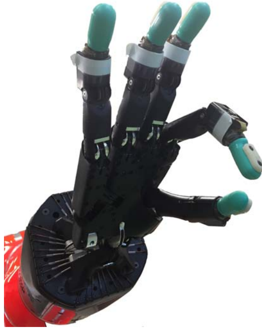
Figure 2.2: An anthropomorphic robot hand: Shadow Hand.
