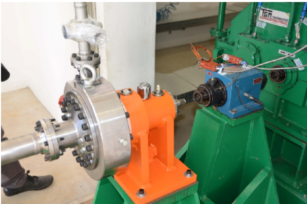
Figure 5. LOX pump test device being installed
