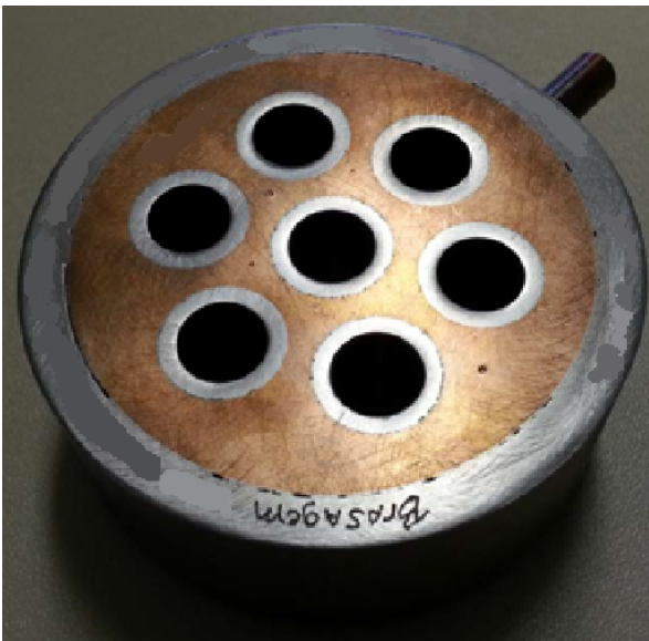
Figure 12. Small-scale injection head brazing model showing the faceplate
