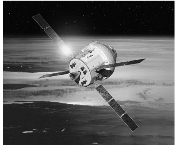
Fig. 4. Artist's Impression of the U.S. MPCV with ESM with Unfolded Solar Arrays. Source: ESA
