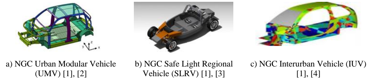
Figure 7 - Body in white concepts and structures for the three vehicle variants
