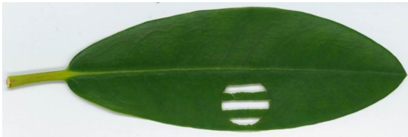
Fig. 1. The holes cut into a broadleaf sample to mimic conifer needle samples set up on the integrating sphere sample port.
