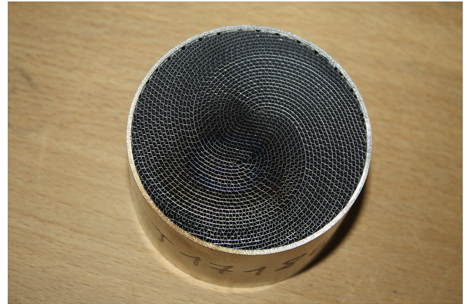
Fig. 3. Receiver test sample ( \varnothing 70 mm) made from a metal honeycomb structure.
