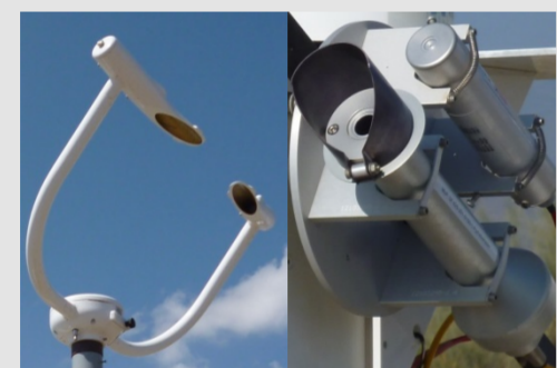
Fig. 2: FS11 Vaisala scatterometer (left), CHP1 Kipp & Zonen pyrheliometer for direct normal irradiance (DNI) measurements (right).
