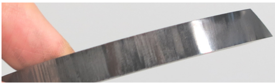
Fig. 16 Piston rings after the test runs
