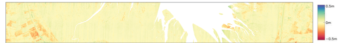
Fig. 36. Difference between F-SAR S- and X-band DEMs, scaled from -0.5 to 0.5 m. The image shows that differences in penetration between S- and X-bands are below a few centimeters for the majority of the scene, and cause the height differences of around 30 cm for areas with short vegetation.
