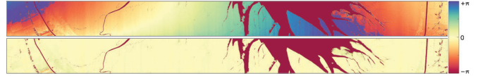
Fig. 16. Rewrapped difference between the X- and S-band phases after calibration (phases scaled to the S-band geometry). (Top) Data set of each acquisition frequency was individually calibrated. (Bottom) DFDB scheme was employed.
