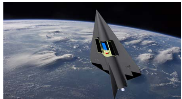
Figure 4: Artists impression of satellite payload release from SpaceLiner 7 Orbiter’s open payload bay in LEO
