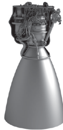
Figure 14: CAD-model of SpaceX’ Raptor engine in 3290 kN variant [12]
