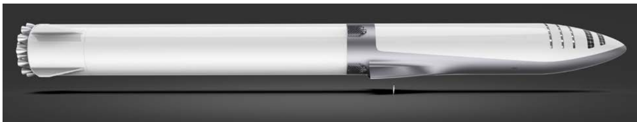
Figure 6: Drawing of BFR launch configuration with passenger stage on the right and booster stage on the left [3]
