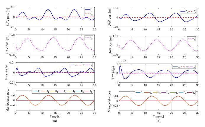
Fig. 8. Simulation results for the tracking case. Left: large and fast trajectory (the 2nd joint travels 90° in the fully stretched configuration). Right: small and slow trajectory (the 2nd joint travels  $15^{\circ}$ ). The maximum deviations of  $r_x$  were about 0.073 m (left) and 0.0046 m (right).
