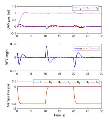
Fig. 5. The manipulator moved while hovering. Although the movement was close to the full swing, stability could be maintained.
