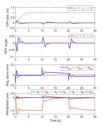
Fig. 7. The proposed controller was applied to UAV-M equipped with the position servo manipulator and angular velocity servo UAV, as shown in Fig. 4. Note that this implementation is almost model-free.  $e_{w,xyz}$  in the third row denotes the tracking error of angular velocity. Despite imperfect reference tracking, stability was maintained.
