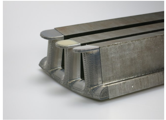
Fig. 13. Metallized winding head support at stator lamination segment.
