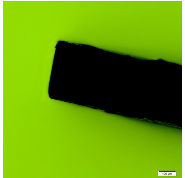
Fig. 6. Light optical microscope image of the laser cutting edge of a 0.35mm stator lamination.
