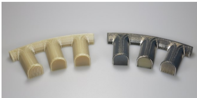
Fig. 12. 3D printed winding head support with (right) and without (left) surface metallization.
