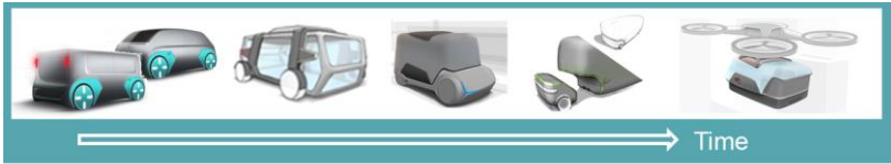
Figure 2: Vehicle concepts with different possibilities to separate driveboards and capsules (own visualization).
