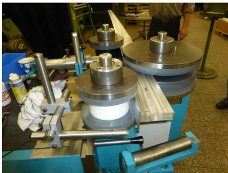
(a) Roll-form production process of the stringers.
