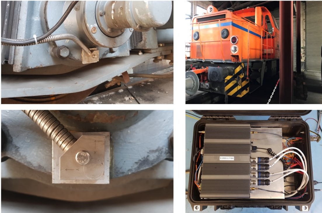
Figure 2: Mounted acceleration sensors on the front axle box of the shunter locomotive (left side, overall view and close up), shunter locomotive (upper right), sensor box without external sensors (bottom right)
