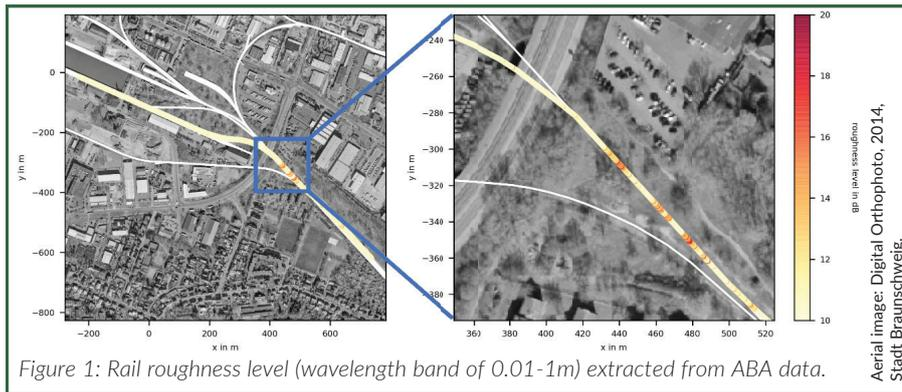
Figure 1: Rail roughness level (wavelength band of 0.01-1m) extracted from ABA data.
