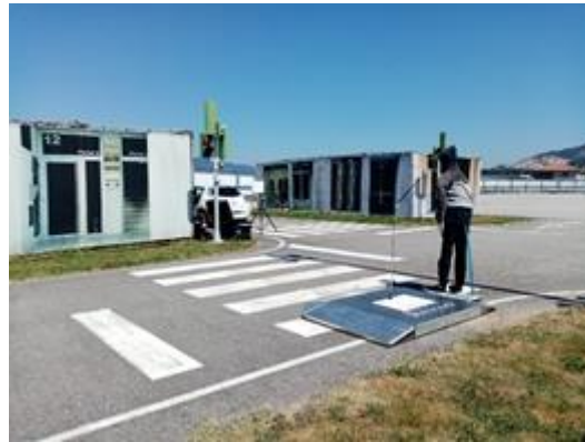
Figure 97: Pedestrian crossing simulation platform during track tests.
