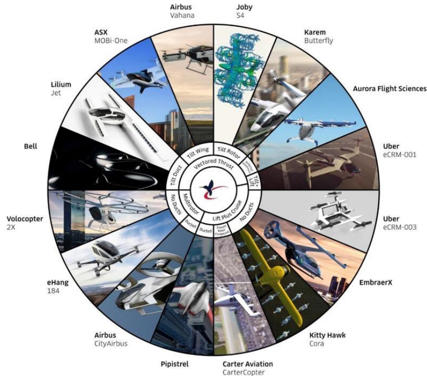
Figure 2.3: Classification of eVTOL Aircraft Configurations by the eVTOL Wheel [21]
