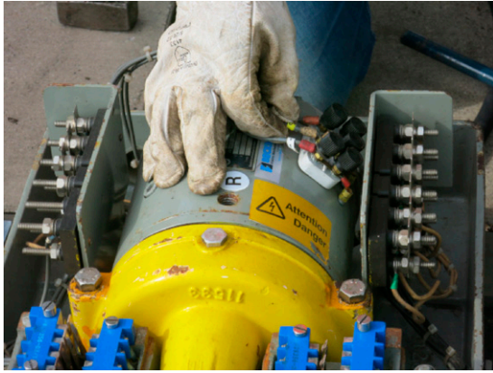
Figure 2. Experimental simulation of a bad contact in the power supply.
