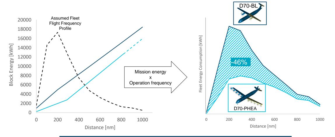
Since the regional fleet mostly operates at lower distances, plug-in hybrid operation can almost cut the operational energy consumption in half.
