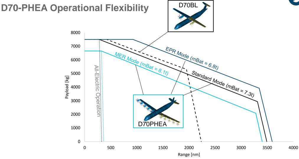
A configurable battery could improve the payload-range flexibility compared to conventional turboprops.
