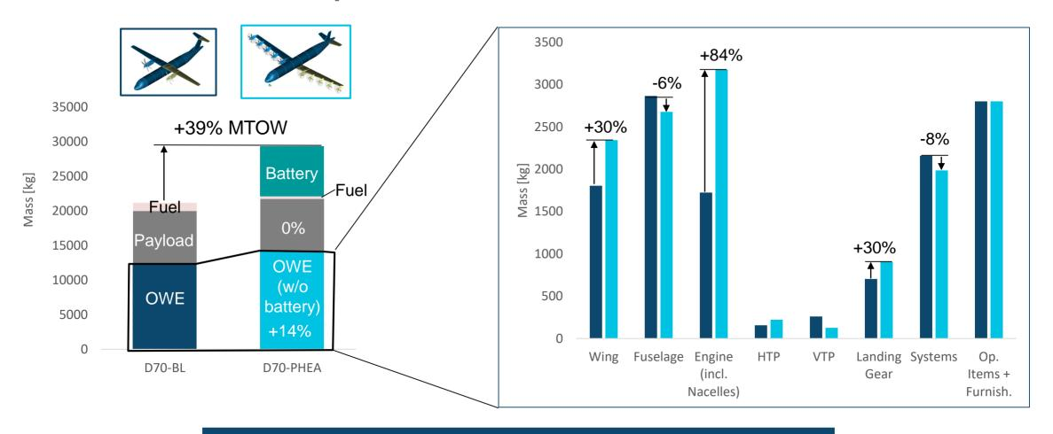
An MTOW increase of 38.5% is mostly due to the heavy battery. The empty mass of the aircraft increases only 14%.
