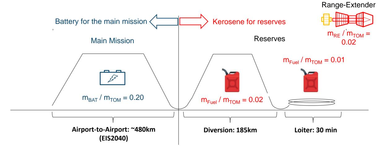
More achievable electric range by using a range extender with kerosene for reserves.
