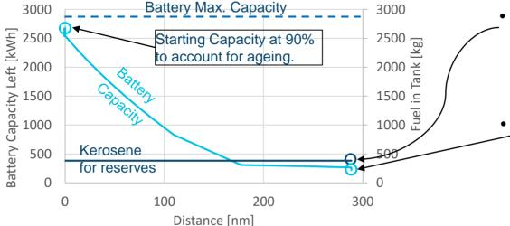
Sufficient fuel is carried in case a diversion after the mission is needed.
