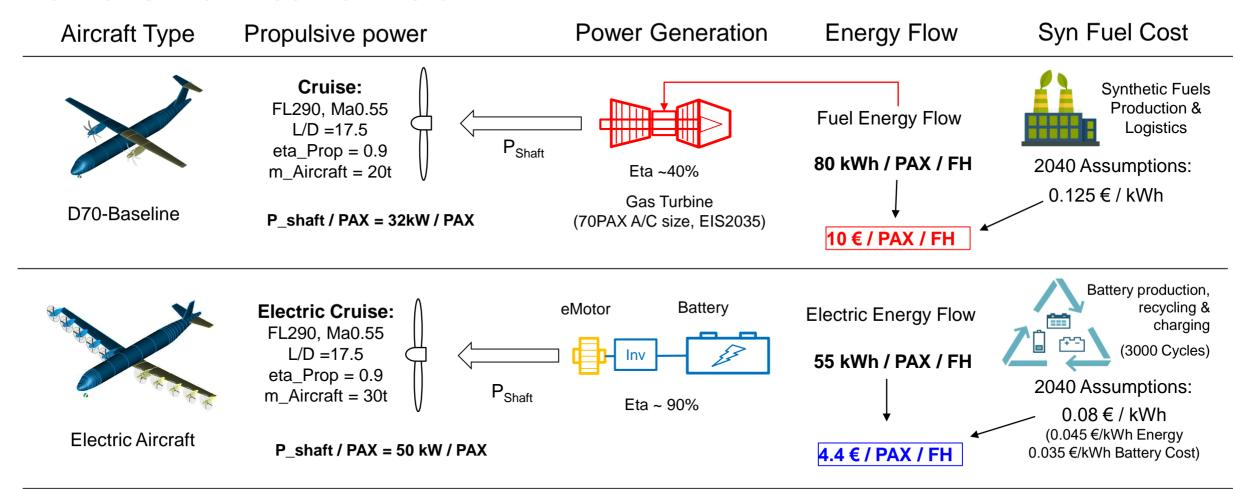
The energy cost for electric flight is potentially ~30% more energy efficient and over 50% cheaper than flying with synthetic fuel.
