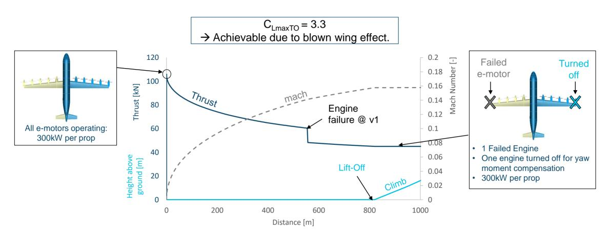
TOFL ~ 1000nm with a requirement of 1500m, with e-motors sized only for sufficient climb power.
