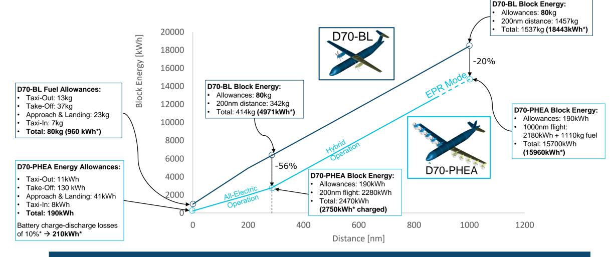
PHEA offers energy savings of around 60% for operation up to 300nm & efficiency improvement even at 1000nm.
