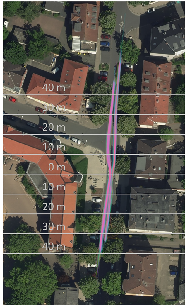
Figure 3: Trajectories of n = 209 encounters ( n = 418 vehicles). Distance to the narrow passage was based on the trajectories’ UTM north coordinate (exemplary distances are shown as grey lines).
