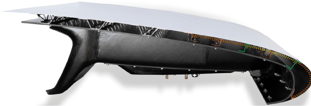
Figure 13 – Possible double layer installation of the coils system (shaded in orange and yellow).
