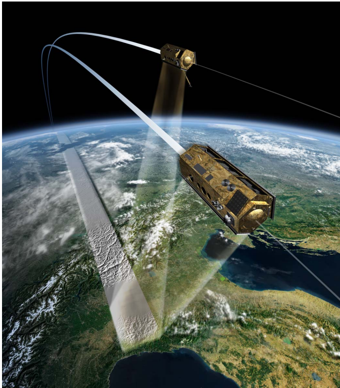
Fig. 13. Artist view of the TerraSAR-X and TanDEM-X satellites flying in close formation. The main goal of the TanDEM-X mission will be the acquisition of a global high-quality DEM with high resolution.
