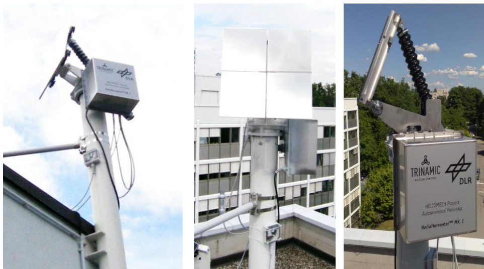
Figure 6: Test heliostat with dummy facets.
