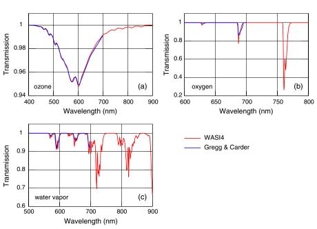
Fig. 1. (Color online) Atmospheric transmission after absorption by ozone, oxygen, and water vapor.
