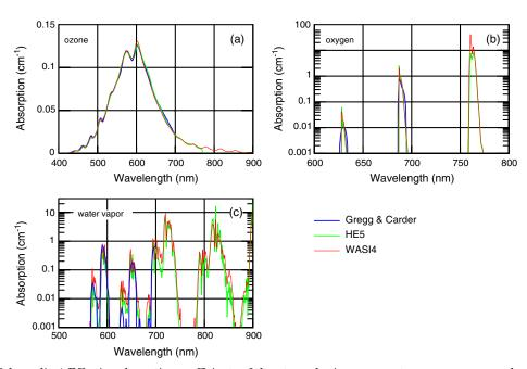
Fig. 2. (Color online) Effective absorption coefficients of the atmospheric components ozone, oxygen, and water vapor.
