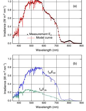
Fig. 10. (Color online) Example for inverse modeling of an irradiance measurement. Fit parameters:  $X=0.85~{\rm g\,m^{-3}},$   $Y=0.21~{\rm m^{-1}},$   $f_{dd}=1.02,$   $f_{ds}=1.02,$   $z=1.06~{\rm m}.$  (a) Measured spectrum and model curve. (b) Direct and diffuse component obtained from inverse modeling.
