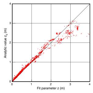
Fig. 3. (Color online) Comparison of analytically estimated sensor depths with results from inverse modeling.
