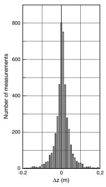
Fig. 13. Sensor depth variability during a measurement.
