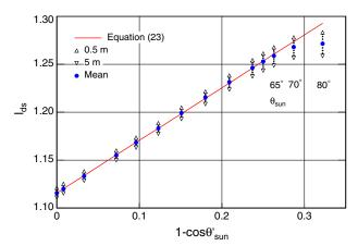
Fig. 7. (Color online) Dependency of the relative path length of diffuse radiation on depth and on the Sun zenith angle.
