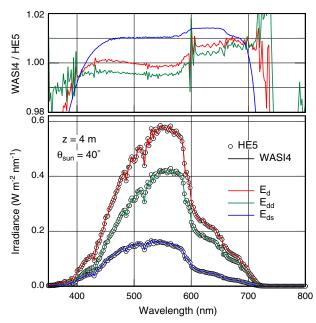
Fig. 8. (Color online) Comparison of spectral shape for WASI4 and HE5 simulations of irradiance.
