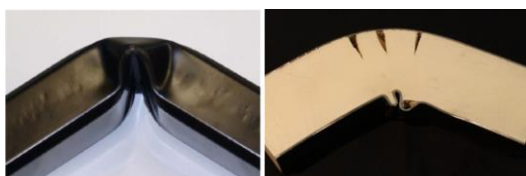
Fig. 6 Formation of fold on compressed side of hollow (left) and PU foam-filled (right) sections
