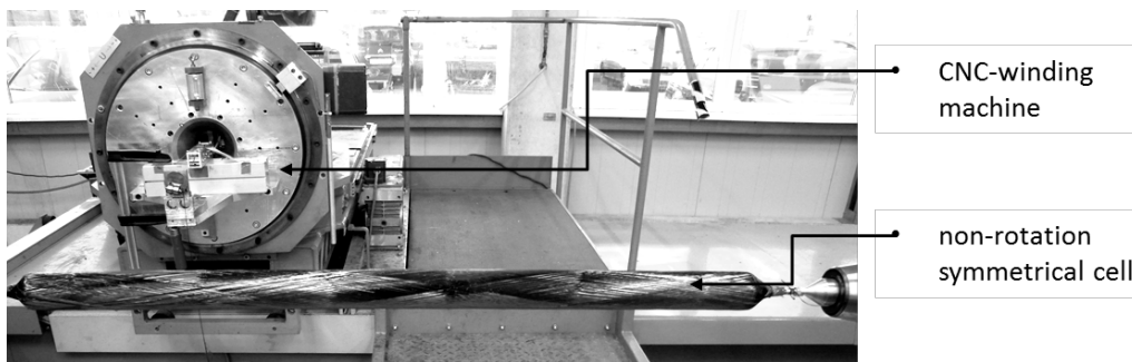
Figure 4. CNC-winding machine with a full wound non-rotationally symmetrical cell
