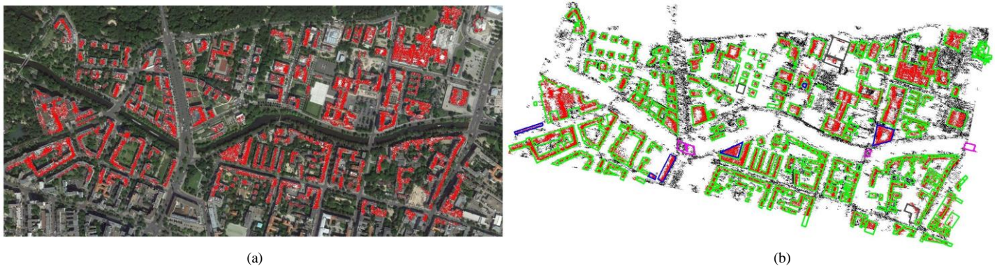
Figure 3. Results of building extraction: (a) Extracted roof points in red are overlaid onto the optical image (© Google) of the area of interest; (b) Red and black points depict building and non building points respectively. The overlaid green polygons are reference buildings downloaded from OSM [12]. Blue polygons are manually extracted buildings not present in OSM data. Gray polygons are newly constructed buildings that are not present in our dataset whereas magenta colored polygons are buildings that do not actually exist but present in OSM data. Both gray and magenta polygons are not included in the evaluation.
