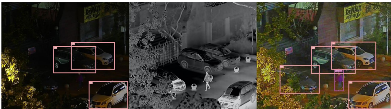
Fig. 6 YOLO performing object tracking on a security camera video on original (left) and VEVid preprocessed images (right). Image from an infrared camera (center) shows that hidden details that are revealed by VEVid match the real scene. S=0.4 , b=0.16 , G=1.4
