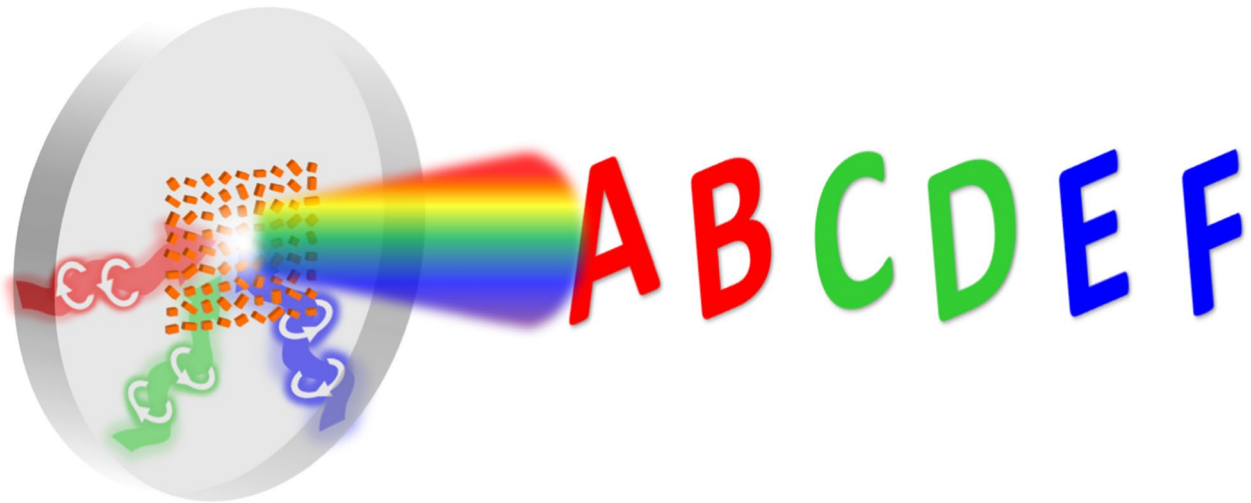
Fig. 1 Schematic of six-channel crosstalk-free holographic image projection over a broad visible range by the spin and angle co-multiplexed waveguide-based metahologram. Each of the six independent images (e.g., capital letters with different colors shown in the schematic) can be selectively projected into the far field when the metahologram is illuminated by a guided incident light with certain spin state and azimuthal angle
