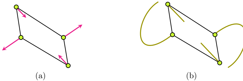
Figure 7.3: A C_2 -symmetric infinitesimal flex of the framework from Example 3.2.1 (a) and the path taken by the joints of the framework under the corresponding symmetry-preserving continuous flex (b).
