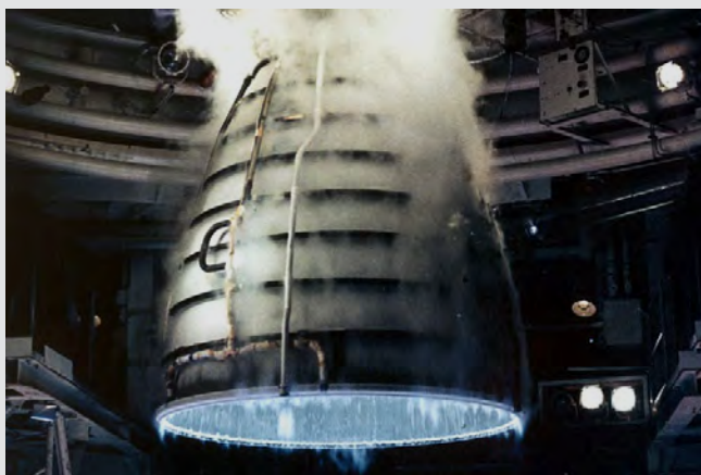
A space shuttle main engine burning hydrogen with oxygen, produces a nearly invisible flame at full thrust. / Nasa, public domain
