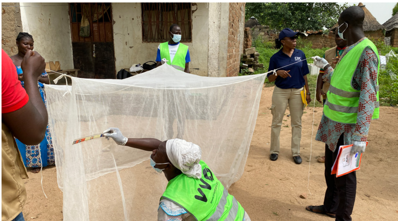
A trained community member checking for holes in a mosquito net after one year of use by a household in Cameroon.
