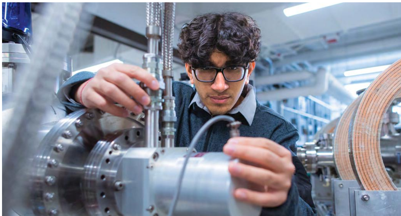
MIT first-year Akarsh Aurora is investigating a special type of thin film tape made of rare-earth barium copper oxide, which is used in the superconductors that drive nuclear fusion, to understand how it behaves when exposed to neutron irradiation. Here he fixes the cryohead of a vacuum-sealed particle accelerator, which will be used to irradiate the tape and help his team glean insights about the material’s thermomechanical properties. Photo: Gretchen Ertl
