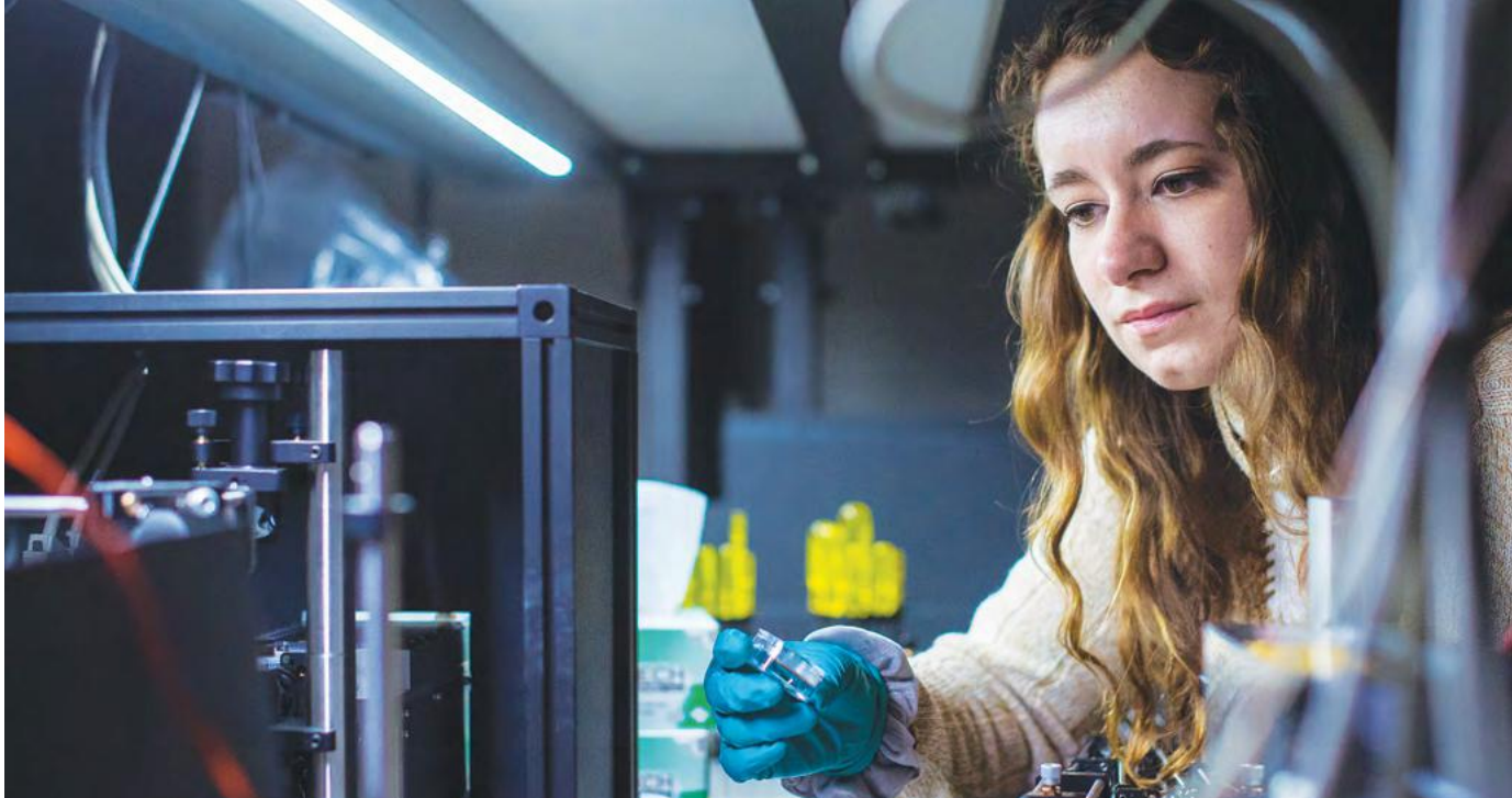
Through the FUSar program, MIT junior Lauryn Kortman measures the material properties of REBCO (rare-earth barium copper oxide), a high-temperature superconductor, before and after being exposed to proton irradiation. Here she analyzes a sample next to a transient grating spectroscopy machine, which can be used to nondestructively measure the bulk modulus, thermal diffusivity, and other key properties of a material. Photo: Gretchen Ertl
