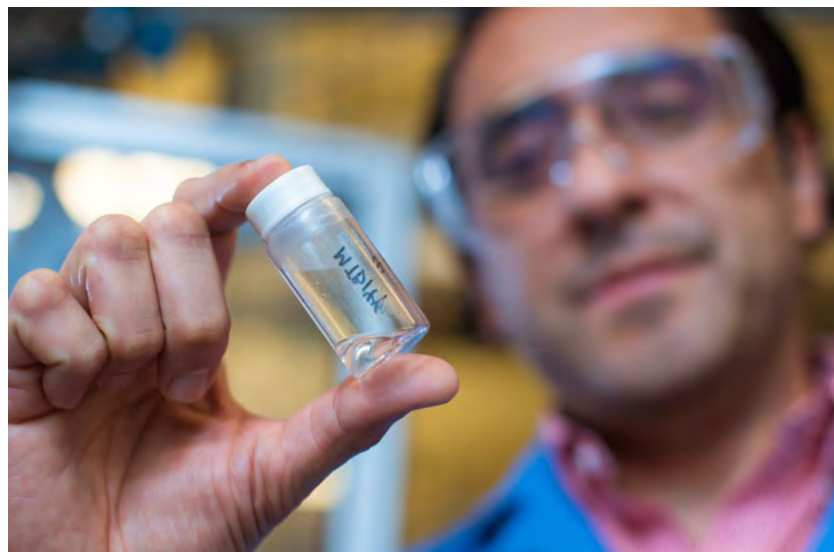
The two vials shown above contain products from key steps in the MIT procedure. The brown lignin oil in the left-hand vial formed when the biomass was exposed to the first catalyst. The clear liquid in the right-hand vial—here displayed by Professor Román-Leshkov—formed when the lignin oil passed through the trickle-bed reactor for the second time. Now free of oxygen molecules, it is the aromatic fraction needed to make today’s aviation fuel 100% sustainable. Photos: Gretchen Ertl
