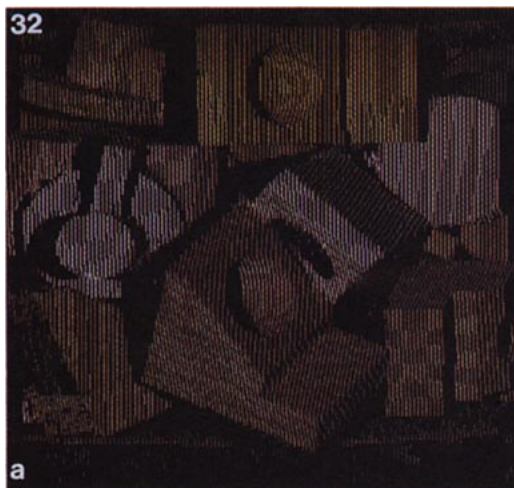
FIG. 26. (a) A scene containing objects from the model-base shown in Fig. 1. (b) Color-composite light-stripe image of the scene. (c) 3D plot of points detected. (d) Segmented image.
