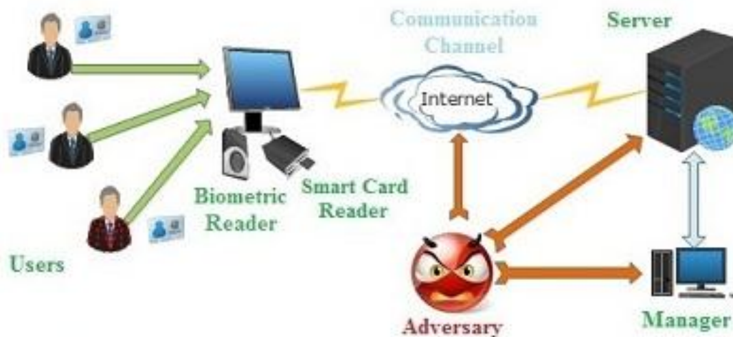
Figure 1. Simplified example of Smart Card based Remote User Authentication Scheme
