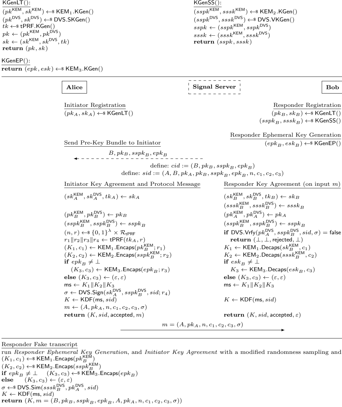
Fig. 8. The SPQR protocol (top: key generation, middle: protocol flow, bottom: fake transcript generation), combining static, semi-static and ephemeral key encapsulation schemes \text{KEM}_1 , \text{KEM}_2 , and \text{KEM}_3 , a designated verifier signature DVS, and a twisted pseudorandom function tPRF.
