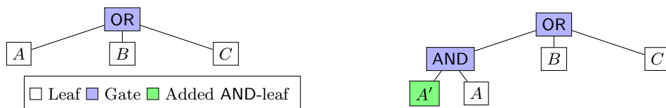
Fig. 6: Access-tree (left-side) and delegated-tree (right-side) where the leaf associated with attribute A is changed into an AND-gate with a new child leaf associated with attribute A'
