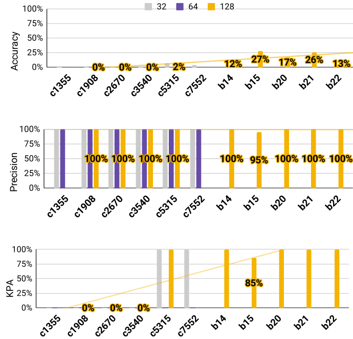
Figure 9: Results for the MuxLink attack on IsoLock Variant I, with both configured for default hop-sizes h' = h = 3 . MuxLink threshold th = 1 . Embedded data points refer to key-size of 128 bits.
