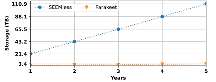
Fig. 13: Comparison of storage costs of Parakeet and SEEMless in the first five years.
